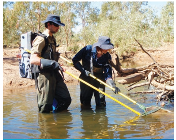
Back-pack electrofishing offers the only practical means to survey waterways large woody debris
