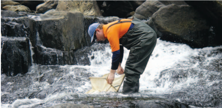
Surber-sampling supports rigorous statistical analysis of data - essential for monitoring
